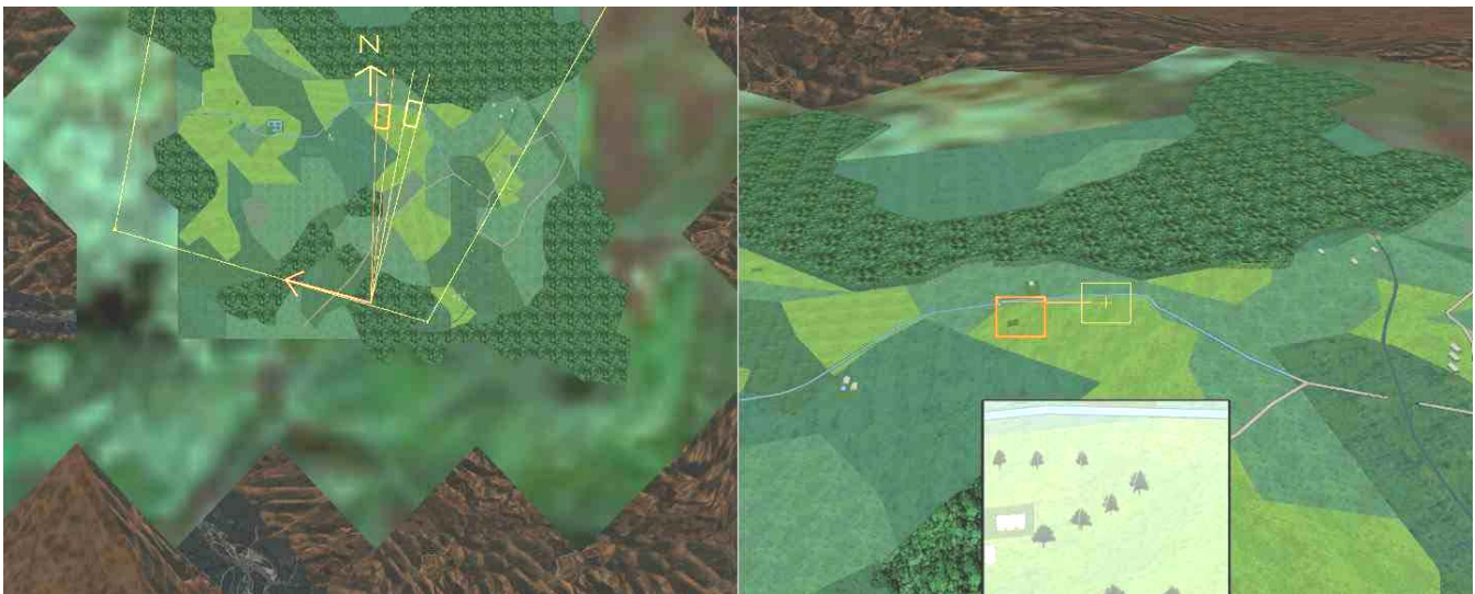
Figure 2: The Left Panel shows the 2D Map with the Position of the UAV in the Center. The right panel shows the 3d map, which is drawn from the viewpoint of the camera. In both displays, the yellow footprint shows the part of the environment that corresponds to the camera image and the orange footprint shows the predicted position. The camera images are presented at the bottom of the right display.
